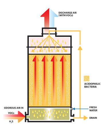
**Bioscrubbers** rely on microorganisms present in water that's recirculated through the treatment vessel. Foul air is forced upward through the bottom of the vessel. On its way up, it's dispersed through synthetic media and contacts the water laden with microorganisms.
