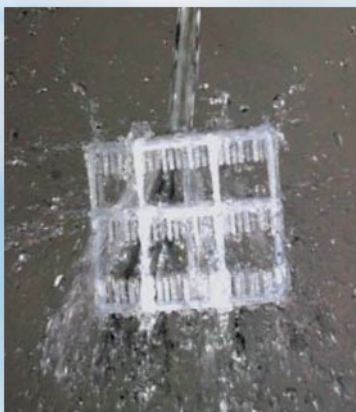
A photograph of liquid dispersion over Qimi's polypropylene media.
